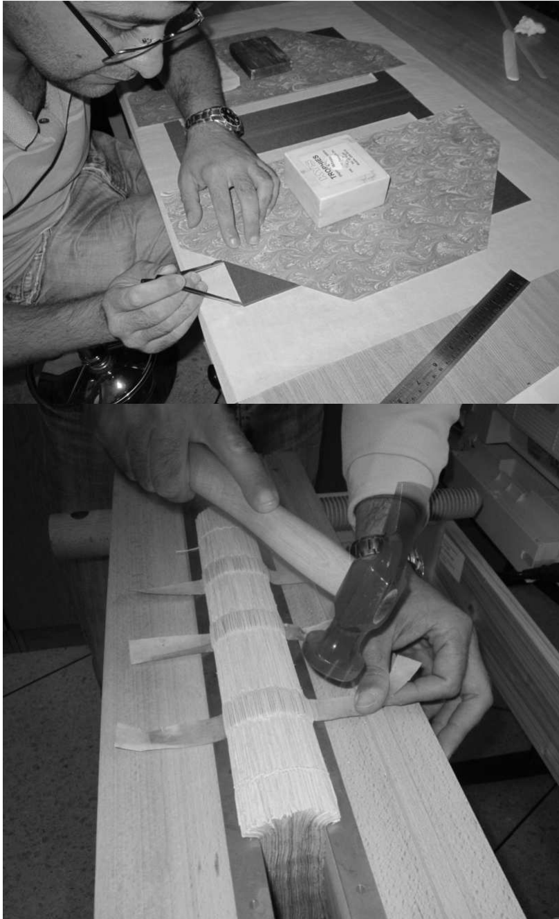
Measuring before gluing on the marble paper—creating of facsimile; Codice DeRohan. Rounding of the Spine after sewing.
